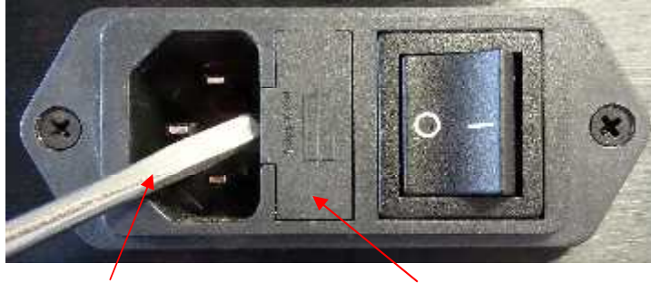
Prying open with small screw driver
