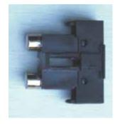
4. Replace fuse holder into power connector by making sure that good fuse is at bottom. Replacement fuses should be rated:
